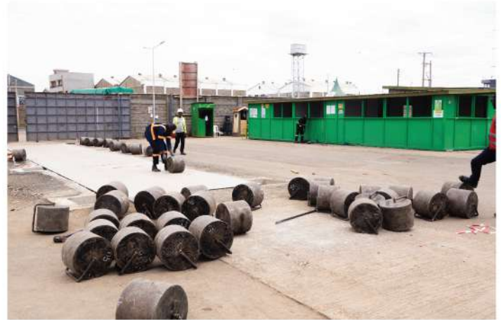
Calibration of the weighbridge
