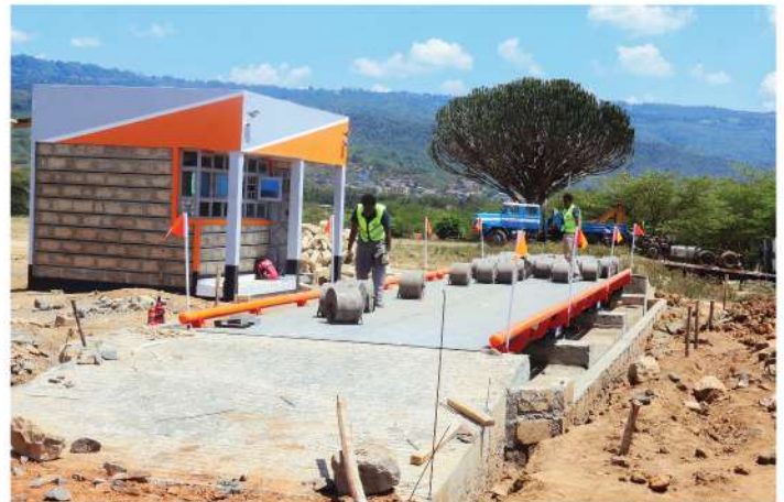
Calibration of the weighbridge
