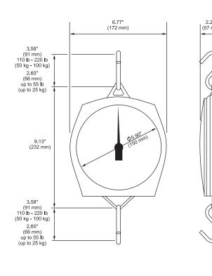
The robust 235 Salter Mechanical Hanging Scales provides high quality, repeatable accuracy. tails. Designed and manufactured to last, the 235 Salter Mechanical Hanging Scales are all made from the highest quality materials and designed to deliver well over one million weighments in the life of the scale. Fitted with precision machined rack and pinions with fully corrosion resistant stainless steel hooks and
